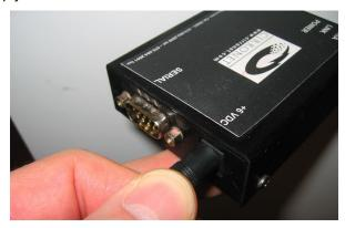
Connect the wall-mount end of the power supply to a wall outlet with either 110VAC or 220VAC. The Power LED on the ZN-241G will come on and after a moment the Data LED will blink. The Data LED blinking means the ZN-241G is looking for another ZN-241G to link to.
