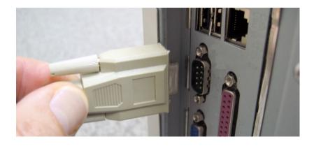
On the other ZN-241G attach the loop-back connector provided as part of the kit.
