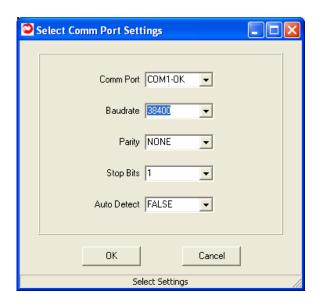
The Select Comm Port Settings dialog is pre-loaded with settings the ZN-241G has when it ships from the factory. In most instances, simply clicking OK will allow ZNWizard to find the radio and load the main program window. If, however, the default settings are incorrect, the radio will not be found. This screen allows you to connect to the radio using two methods.
