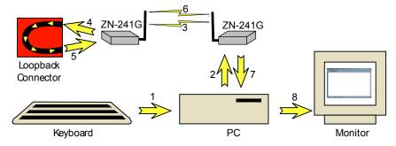
Congratulations! You have just set up a wireless network. You can remove the loop-back connector from the ZN-241G and connect it to a device with a serial port using the second serial cable provided. Refer to the information on the device for steps to set the devices serial port data rate to 38400.
