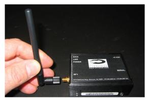
If the folding part of the antenna is not in the right position to stick up above the ZN-241G, hold onto the knurled bottom of the antenna and twist the upper part of the antenna until the foldable part of the antenna sticks up above the ZN-241G. DO NOT TWIST THE ENTIRE ANTENNA AS THIS MAY DAMAGE THE ANTENNA.
