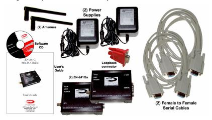
The ZN-241G radio is a simple-to-use, simple-to-setup wireless networking device. With its Auto-Config mode, all that is needed to send data between two ZN-241Gs is to attach the antennas, connect the radios to serial ports and plug in the power supplies. Each step is described below.
