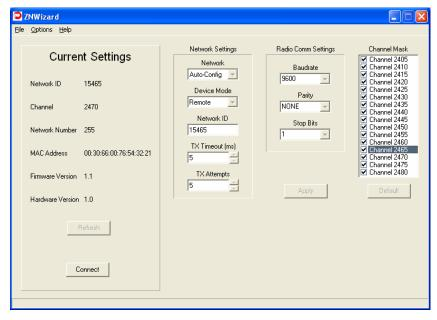
This is the main ZN Wizard program window. On the left side is a readout of the current settings for the radio. On the right side are radio parameters that can be modified. The parameters are grouped according to function.
