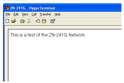
**Note:** If you press the Enter key, Hyper Terminal will move the cursor to the start of the line but will NOT move it down the screen. Any keys then typed will overwrite the previously typed characters on that line. This is the way Hyper Terminal works and is not a problem with the radio. If you want, consult Hyper Terminal's Help files on how to have Hyper Terminal send a line feed when the Enter key is pressed.
