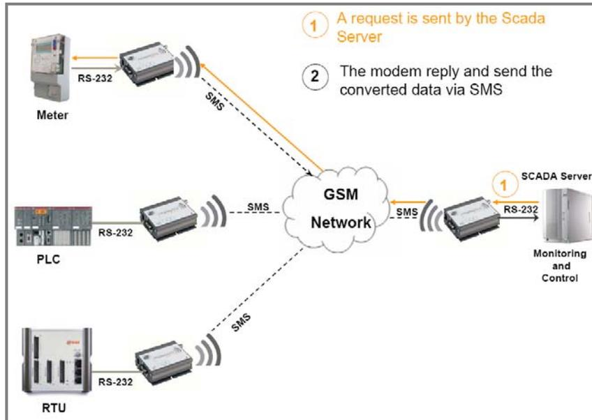
This configuration can be set up on all SCADA protocols and is totally transparent.
