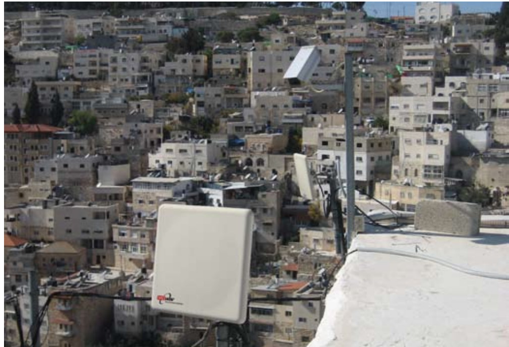
WinLink 1000 deployed for video surveillance transmission
