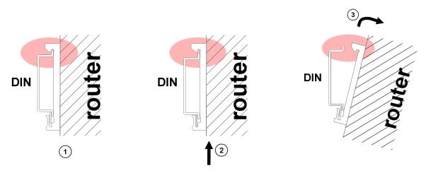
Figure 14: Removal of the DIN Rail
