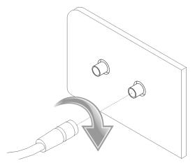
Figure 18: Connecting the antenna
