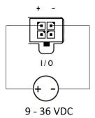
Figure 17: Circuit example – connection of power supply 18
