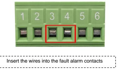
**[NOTE]** The wire gauge for the terminal block should be in the range between  $12 \sim 24$  AWG.
