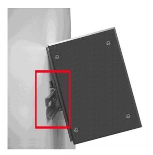
2. Then, lightly push the DIN-Rail into the track.
