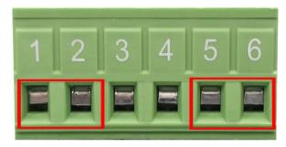
1. Insert AC or DC power wires into the contacts 1 and 2 for power 1, or 5 and 6 for power.
