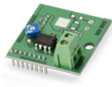
EA2 - audio output module with amplifier
