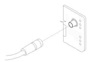
Figure 31: Connecting the antenna
