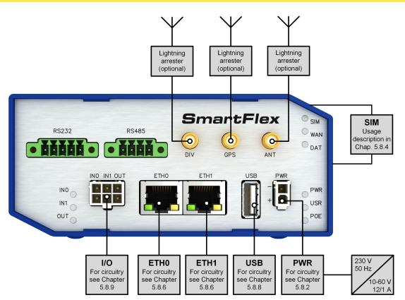
Figure 55: Router connection
