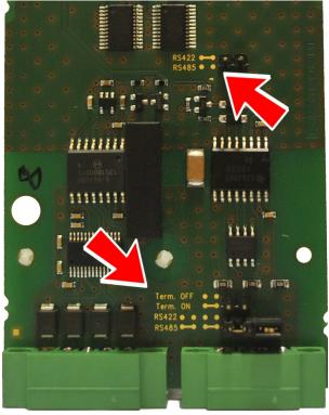
Figure 49: Connection of jumpers
