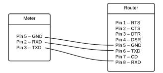
Figure 45: Meter connection to router
