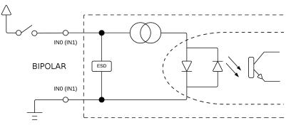
Figure 40: Binary inputs connection
