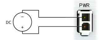
Figure 30: Connection of power supply
