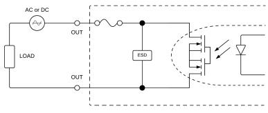
Figure 41: Binary output connection
