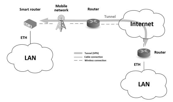
Figure 3: Using VPN tunnel
