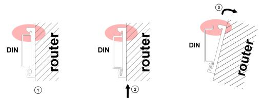
Figure 27: Removal of the DIN rail
