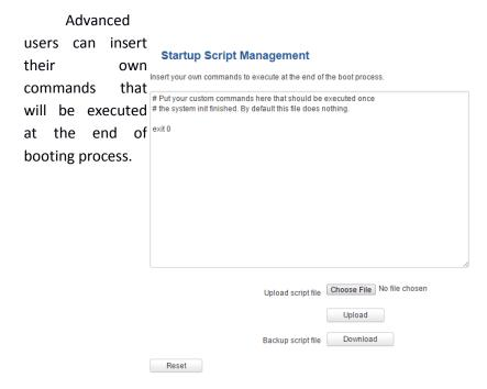
In *Script Management* window is shown content of a file /etc/rc.local. This file is executed at the end of startup, executing the line: sh /etc/rc.local In this script is needed to use sh (ash) commands. It should be noted, that this is embedded device and sh functionality is not full.
