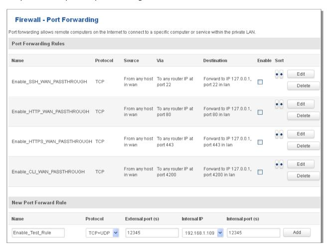
You can use port forwarding to set up servers and services on local LAN machines. The above picture shows how you can set up a rule that would allow a website that is being hosted on 192.168.1.109, to be reached from the outside by entering <a href="http://routersExternallp:12345/">http://routersExternallp:12345/</a>.
