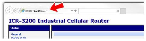
Figure 23: Entering the IP address of the router
