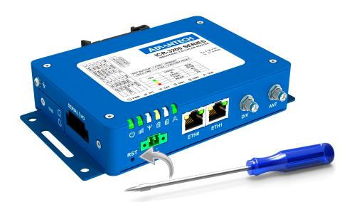
Figure 18: Router reset
