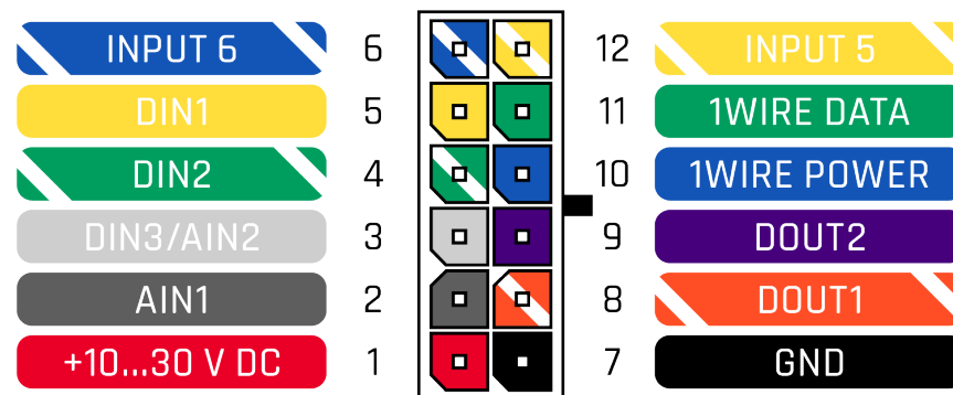
Figure 2 FMB122 2x6 socket pinout
