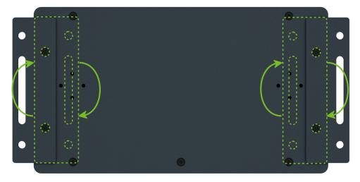
Figure 7: Rotated Wall Mounting Clips
