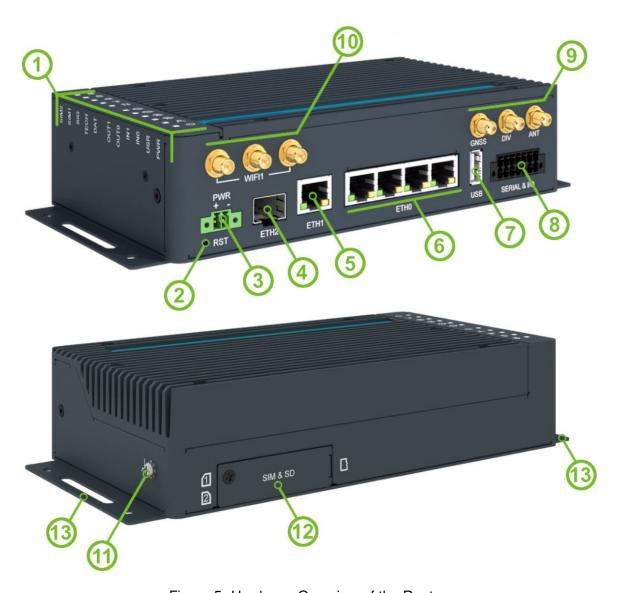
Figure 5: Hardware Overview of the Router
