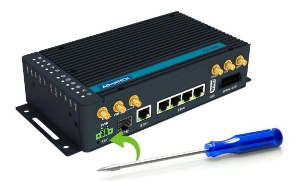
Figure 14: Resetting the Router
