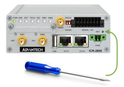
Figure 20: Resetting the Router
